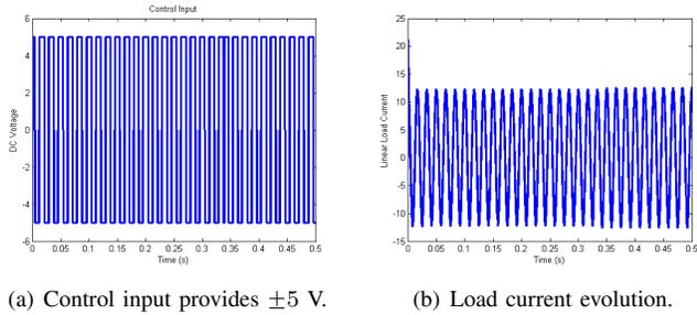
Fig. 4. Control input is  $\pm V_{dc}$  while the load current is a pure cosine since we have a linear load connected to the  $L - C$  filter.
