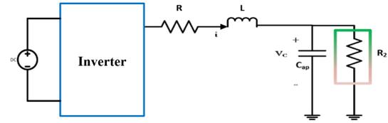
(b) Voltage source inverter filtered by an  $L - C$  filter connected to a linear (resistive) load.
