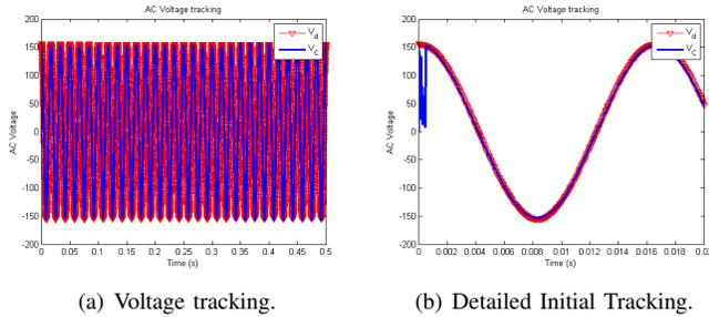
Fig. 3. AC Voltage with a magnitude of  $110\sqrt{2}$  Volts and a frequency of 60 Hz is produced at the output.
