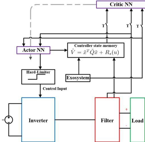
Fig. 2. Visualization of the proposed control architecture for a voltage source inverter where  $T$  represents how fast we are taking measurements of the exosystem and the voltage and the current of the filter by opening and closing three switches. Note that the dashed line shows that the actor is being tuned based on the performance which is computed by the critic NN.
